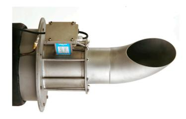
The SEWER-MAG $^{\text{TM}}$  is an insertable full bore electromagnetic flow meter sensor. It ensures extremely accurate flow determination even under difficult flow conditions. The Sewer-Mag is usually temporarily installed in sewer networks to verify or calibrate existing flow meters.
